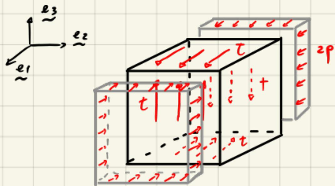
$$\underline{f}_1 = -2p \underline{e}_1 + T \underline{e}_3 \text{ su } \partial C_1.$$
